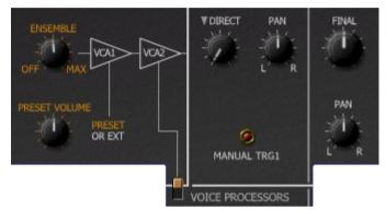
while the *Direct* knob controls the volume of an additional outlet of the polyphonic signal i.e. a mix of all voices after the lowpass filters but before the Equalizer/Resonators section. This is because the original PS-3200 offers two mono outputs, namely the *Final* and the *Direct* signals. On the FB-3200 you can pan both signals individually (see *Tweaks* section) which gives a bit more flexibility.
